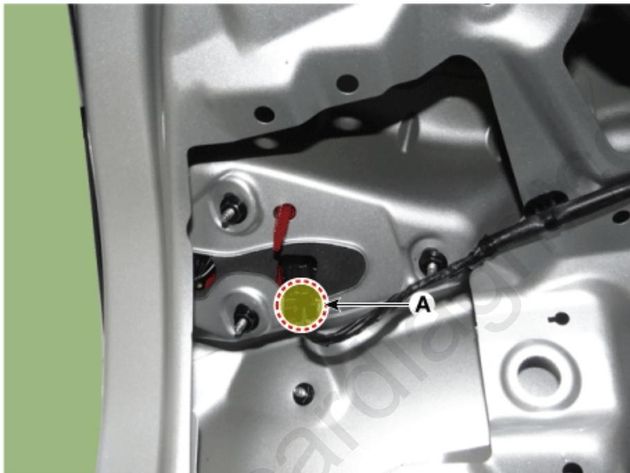
3. Remove the rear combination lamp [inside] (A) after loosening the mounting nuts.
