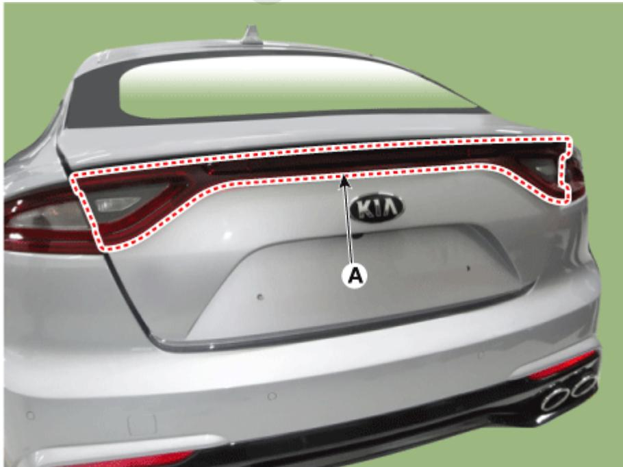
4. Remove the tailgate back panel (A) by using a remover.
